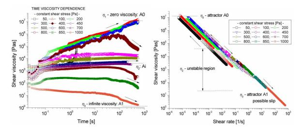
Time dependence of viscosity function and viscosity function vs. shear rate for a lubricated grease based on lithium soup. The experiments are performed in creep tests and evidence the presence of two stable attractors (A0-zero shear viscosity and A1-infinite viscosity) and an unstable region, where the viscosity values are not reached in the limit of infinite experimental time.
